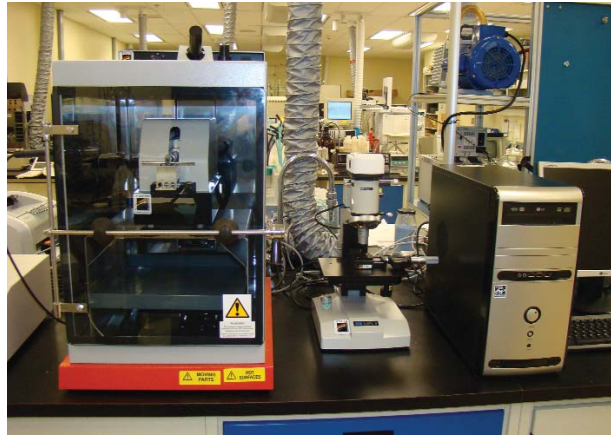
The rig is housed in a temperature- and humidity-controlled cabinet (left). The microscope (centre) is used to view and measure scuff marks on the steel disc.
